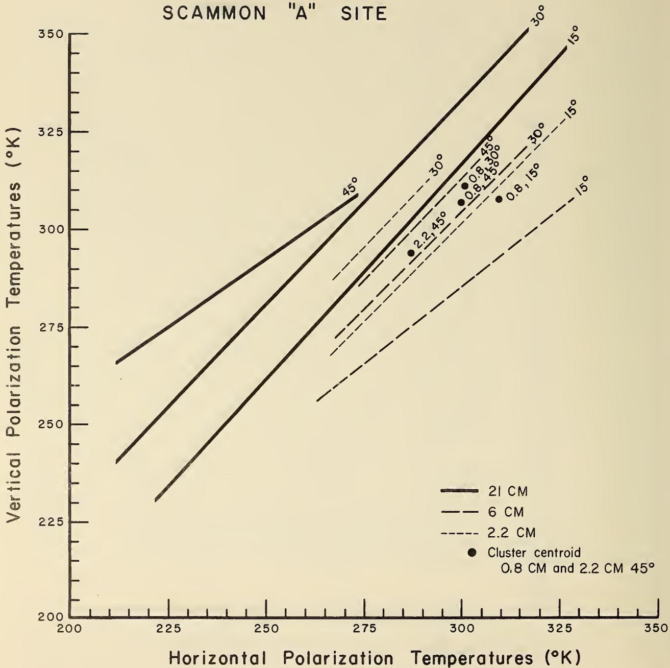
Figure 4.5 Comparison of Vertical and Horizontal Polarizations for All Scammon A Microwave Sensors (Runs 001, 003, and 006).
